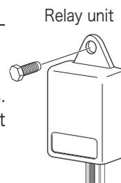
**5** Connect the spade terminal attached to the tip of the black cord (Item ⑧) Then ground it by attaching it to the battery terminal or the vehicle's ground point. (Make sure to properly ground it)
